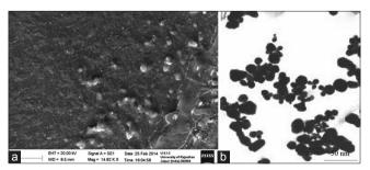
Fig. 2: Micrograph of biosynthesized gold nanospheres. (a) scanning electron microscopy image, (b) transmission electron microscopy image
