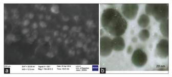
Fig. 1: Micrograph of biosynthesized silver nanospheres. (a) SEM image, (b) TEM image
