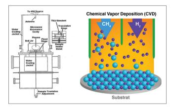
Fig. 9: Chemical vapor deposition method
