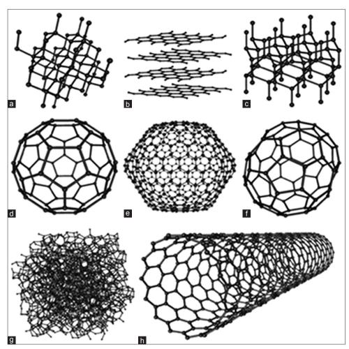
Fig. 3: (a) Diamond, (b) graphite, (c) lonsdaleite, (d-f) fullerenes (C60, C540, C70), (g) amorphous carbon and (h) carbon nanotube
