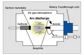
Fig. 7: Arc discharge method
