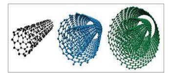
Fig. 2: Single-walled carbon nanotube (CNT), double-walled CNT, and triple-walled CNT
