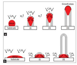
Fig. 6: Growth mechanism of carbon nanotube
