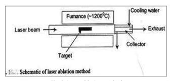
Fig. 8: Laser ablation method
