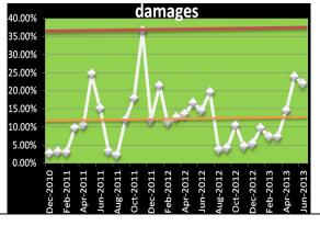
Fig. 11: p-chart for Damages in outlet W
