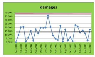
Fig. 3: p-chart for Damages in outlet S1
