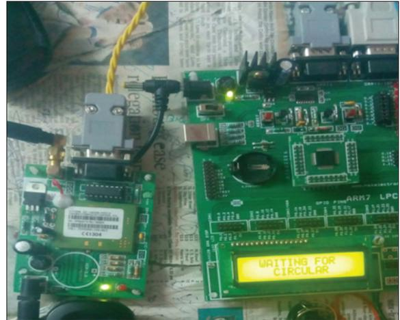
Fig. 3: Interface with global system for mobile module
