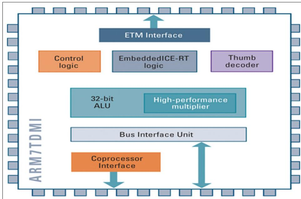
Fig. 1: ARM7TDMI processor architecture
