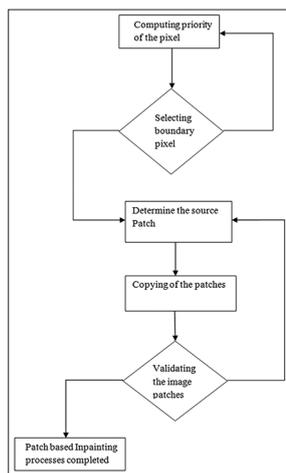
Fig. 3: Flow of greedy-patch based algorithm
