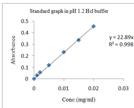
Fig. 1: Calibration curve of Propranolol Hcl in 0.1N HCl Buffer
