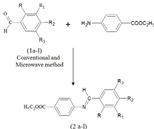
Scheme 1: Synthesis of Schiff bases from Ethyl 4-aminobenzoate
