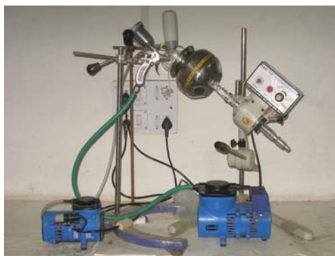
Fig. 1: Photograph of Fabricated Spray Pan Coater
