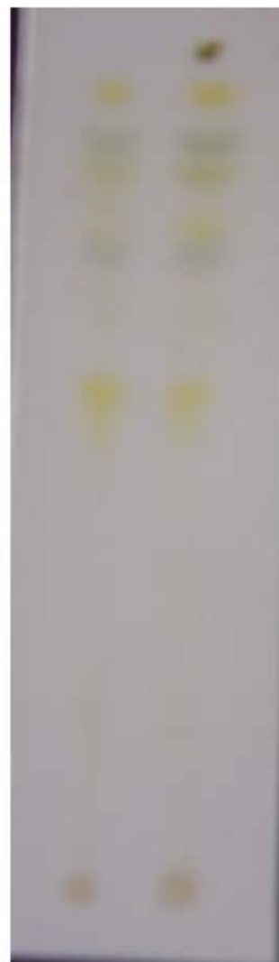
Fig. 6: Chromatogram pattern of n-hexane extract of Kepel leaves on the visual detection. The thin layer chromatography system was silica-gel as stationary phase and the mobile phase system of n-hexane:ethylacetate (1:1)
