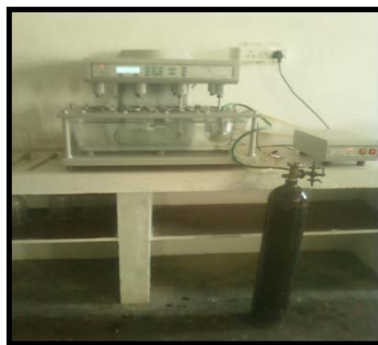
Fig 1: In-vitro drug release study in presence of RCC by USP dissolution test apparatus 1.
