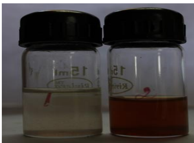
Figure 1: 1-1mM Silver nitrate solution, 2-the color changes to brown after the microwave irradiation
