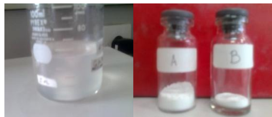
Figure 2: Left to right: hydroxyapatite preparation; result (A = hydroxyapatite synthesis, B = commercial hydroxyapatite)
