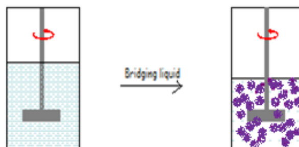
Figure 1: Formation of spherical agglomerates and separate from the suspending liquid by the addition of a small amount of bridging liquid.
