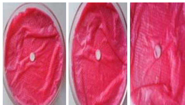
Fig 1: Wetting time of Kollidon CLM (20%) at 5 (a), 25 (b) & 33 (c) Seconds.
