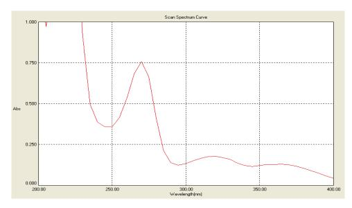
Fig.1: UV spectra of a mixture of HCTZ (270 nm) and AB (365 nm) (10  $\mu g/ml$  each)
