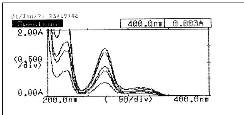
Fig. 2: Spectra of HCT in urea as hydrotropic agent
