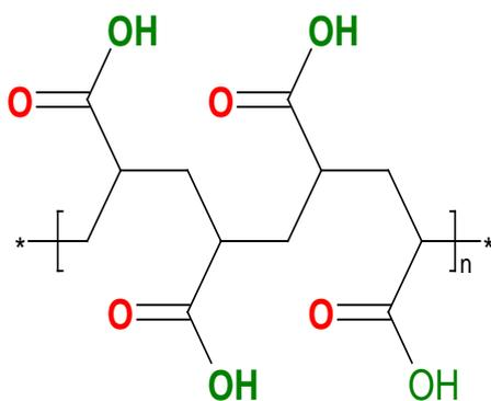
Fig. 2: Structure of Carbopol Polymer (Polyacrylic acid)
