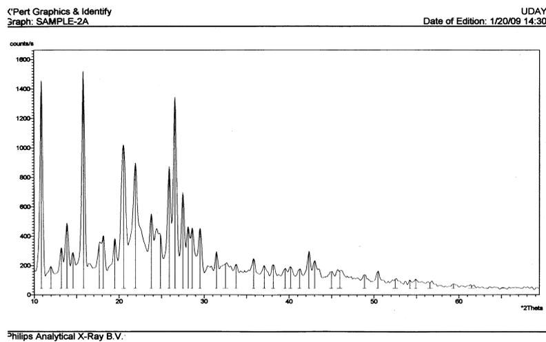
Fig. 11: X-ray diffraction patterns of Mucoadhesive Suspension
