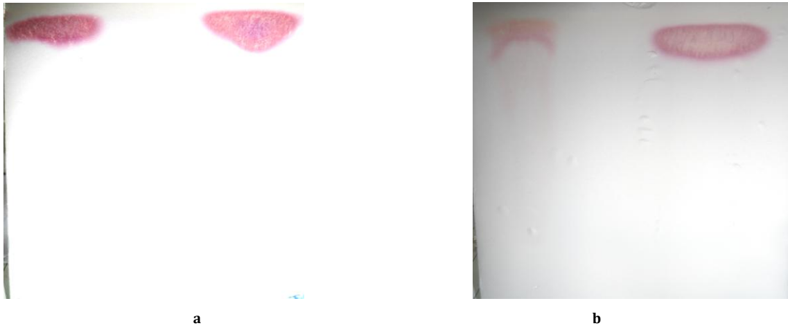
Fig. 4: Amino acids standards: a- left to right showing isoleucine and leucine & b- left to right showing cystine and amino butyric acid.
