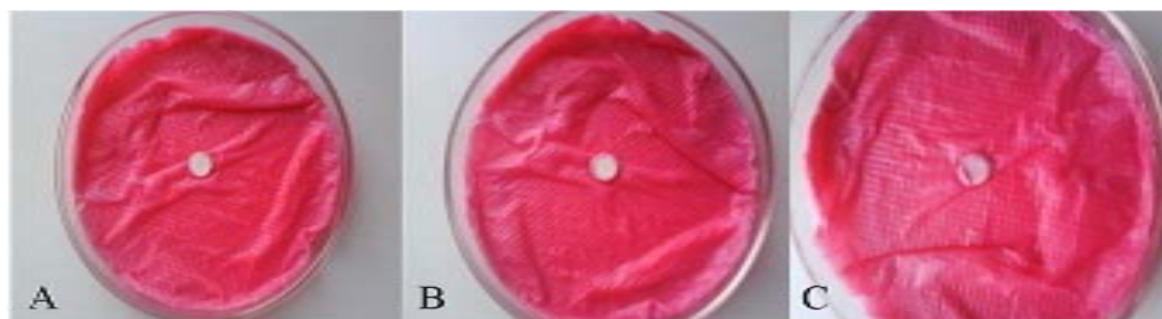
Fig. 2: State of Tablet while measuring Wetting Time (A) Initial stage, (B) Intermediate, (C) Completely Wetted Tablet
