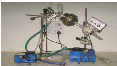
Fig. 1: Fabricated coating pan for coating of ciprofloxacin tablets
