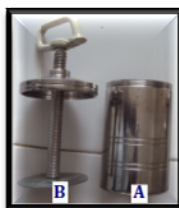
Fig. 2: A. Cylindrical steel Barrel, B. Steel conveyer
