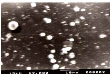
Fig. 7: Scanning electron microscopic photograph of drug loaded transdermal patch ECP-1. (EC:PVP 5:1) before in vitro skin permeation
