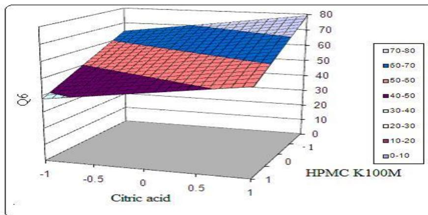
Fig. 5: Response surface plot for Q<sub>6</sub>
