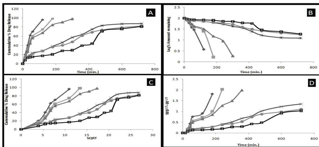
Fig. 5: Dissolution Graphs (N=3) (A) Zero order Model (B) First Order Model (C) Higuchi Model and (D) Hixon-Crowell model comparing six formulations, — F1, — F2, — F3, — F4, — F5 and — F6
