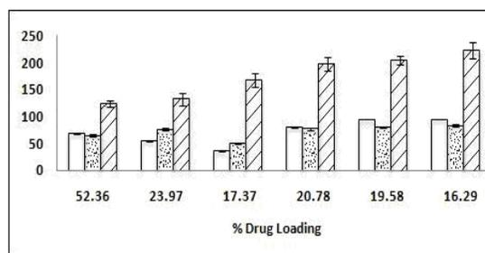
Fig 4: Bar graphs showing effect of % Drug loading on □ % Encapsulation efficiency, ▨ % Batch yield and ▩ particle size of LP microspheres
