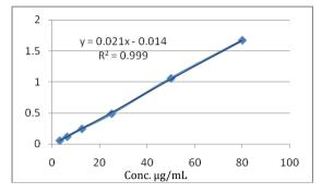
Fig. 2: Standard plot for Gliclazide
