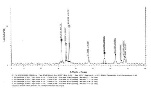
Fig. 2: XRD of Zinc oxide nanoparticle (1, 2 Ethanediol medium)
