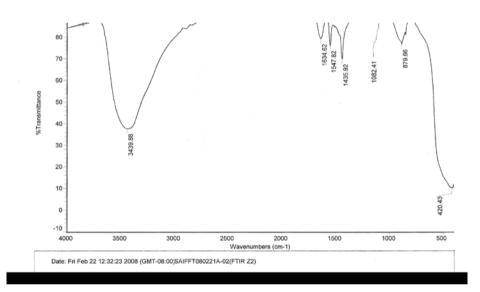
Fig. 4: FTIR of Zinc oxide nano particle (1, 2 Ethanediol medium)
