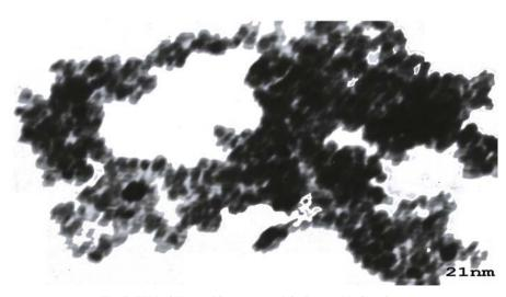
Fig. 5: TEM of Zinc oxide nanoparticle (water Medium)
