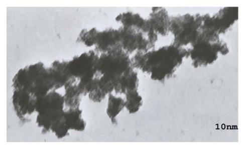
Fig. 6: TEM of Zinc oxide nanoparticle (1, 2 Ethanediol Medium)
