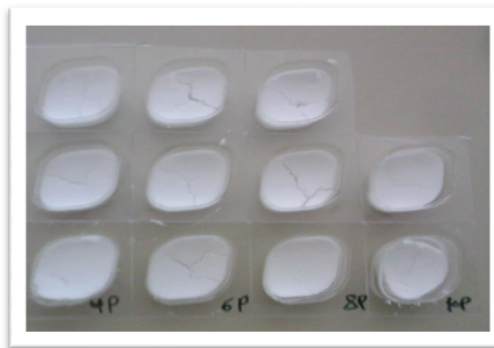
Fig. 1: Photos of crashed oral lyophilizates prepared using the formulas 4P, 6P, 8P and 10P.
