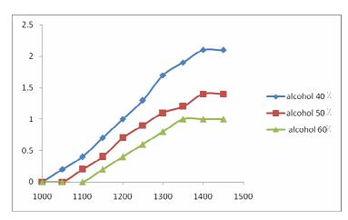
Fig. 3: Polarogram of curcumin at various % of ethyl alcohol in acetate buffer (pH 6)
