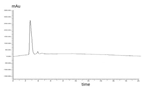
Fig. 4: Typical chromatogram of blank plasma sample
