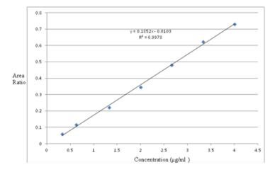
Fig. 6: Calibration Curve of Vildagliptin
