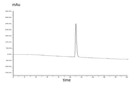
Fig. 2: Typical chromatogram of Vildagliptin (RT-11.2min)
