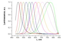
Fig. 2: Fluorescence spectra of CdTe quantum dots of various sizes<sup>12</sup>
