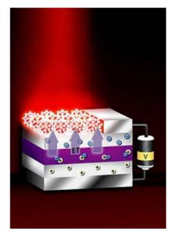
Fig. 3: Wireless device that efficiently produces visible light, through energy transfer from thin layers of quantum wells to crystals above the layers <sup>44</sup>.
