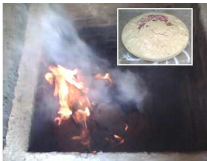
Fig. 2: Photograph of 'puta' in progress. The inset shows the arrangement for puta with cakrikas placed inside earthen bowls with interface sealed by clay-smeared cloth
