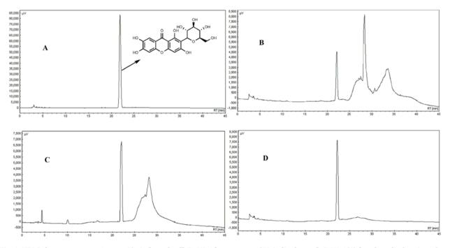
Fig. 4: HPLC chromatograms: A; mangiferin [standard], B; MI-1 [aq. extract of *M. indica* leaves], C; MI-1(1) [methanolic fraction of aq. extract of *M. indica* leaves] and D; mangiferin [isolated from *M. indica* leaves]
