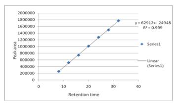
Fig. 4: It shows Calibration curve of Norfloxacin by HPLC
