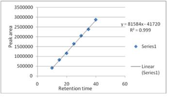
Fig. 3: It shows calibration curve of Metronidazole by HPLC
