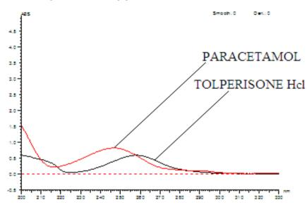
Fig. 2: Overlain spectrum of a mixture of standard Tolperisone HCl and Paracetamol
