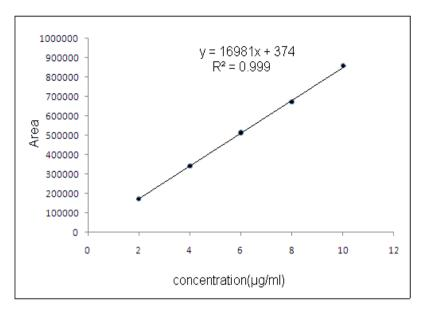
Fig. 3: Calibration curve of Tolperisone HCl
