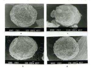
Fig. 1: Scanning electron micrographs of Aceclofenac microcapsules MC1 (a), MC2 (b), MC3 (c) and MC4 (d).
