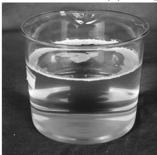
Fig. 1: Floating behavior of Hollow Microspheres in 0.1 N HCl containing Tween 80 (0.02%) after stirring for 12 h.
