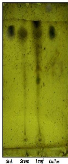
Fig. 4: Thin Layer Chromatogram of G. asiatica plant parts against Quercetin Reference
