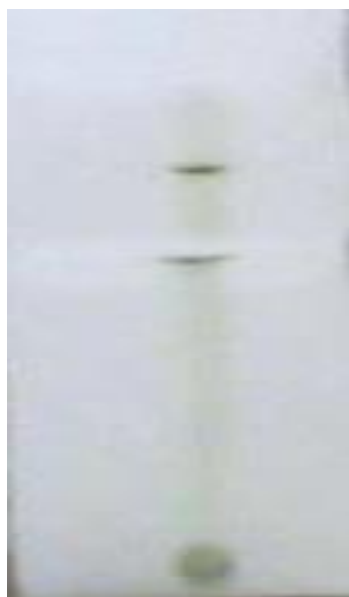
Fig. 1: TLC of Chloroform extract of S. indicum by using solvent system of Acetic acid: Ethanol (1:3) and Detecting agent: Dragendroff's reagent
