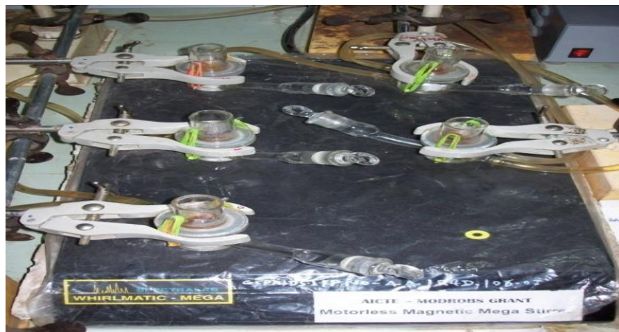
Fig. 2: Assembly for in vitro permeation studies
