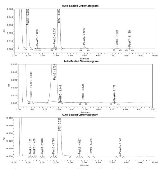
Fig. 3: Auto-scaled Chromatogram A. acid degradation B. base degradation C. oxidative degradation
