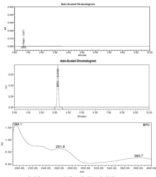
Fig. 2: Chromatograms of A. dilent as blank B. standard C. UV spectrum
