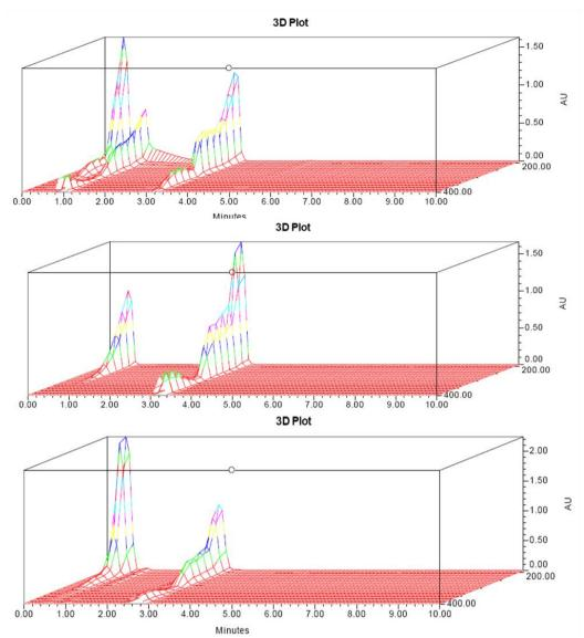
Fig. 4: 3D plots of typical chromatograms of A. acid degradation B. base degradation C. oxidative degradation
