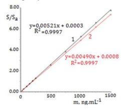
Fig. 2: Calibration curves of GC- ECD determination Di in standard solutions (1) and standard solutions in tomato samples after extraction (2) by the ratio S/ Sa (S- the peak area of Di and Sa - the peak area of the internal standard).
