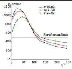
Fig. 3: Effect of spraying time (at 08.00, 17.00 and 21.00 h) on quantity of residual Dimethoate in tomato samples using GC analysis (t,h- is sampling time after spraying by hour ).
