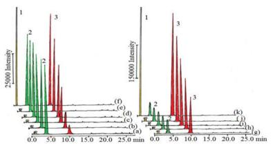
Fig. 1: Chromatograms of Dimethoate (3) in standard solutions in acetone for standard concentrations: a- 25, b- 50, c- 100, d- 150, e- 200, f- 250, g- 500, h- 750, 1000, j- 1250 and k- 1500 ng.mL<sup>-1</sup>(1- Acetone, 2- Internal standard of 1-Chloro-4-fluorobenzene 50 ng.mL<sup>-1</sup>).
