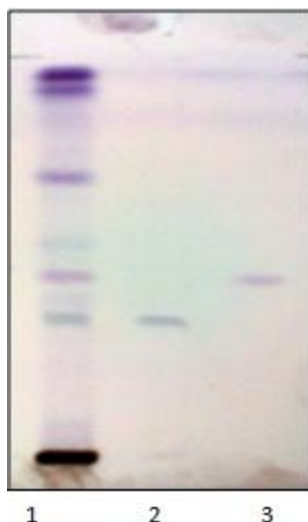
Fig. 1: HPTLC plate showing separation of methanolic extract of dried stem bark powder of Mimosa elengi Linn. (1), standard ursolic acid (2) and standard betulinic acid (3)
