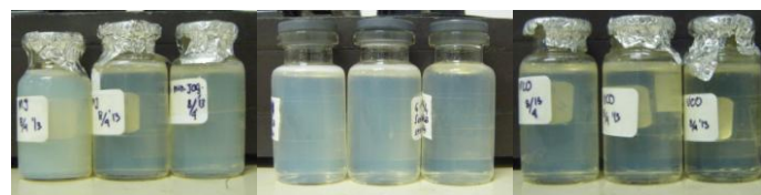
Fig.7: Emulsions used soybean oil (a), corn oil (b) and VCO (c) with surfactants-cosurfactants ratio of 5:1; 6:1; 7:1 and surfactants combination to produced HLB 14.
