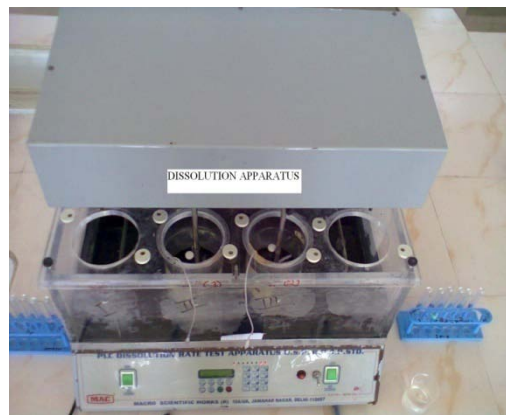
Fig. 7: A photograph taken during the in vitro dissolution study of formula (F6) in a USP TYPE II apparatus.
