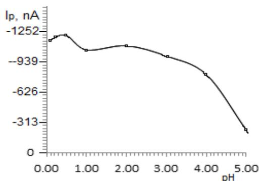
**Fig. 2: The effect of pH solution on  $I_p$  of RSV(9.63 µg.mL<sup>-1</sup>) using DPPA at DME (Purge gas N<sub>2</sub>, Purge time 200 s, Scan rate 6.6 mV/s, U. amplitude -60 mV, t. meas. 20 ms, t. pulse 60 ms, t. step 0.9 s, Temperature of solution 25± 5°C and buffer 0.075 mol.L<sup>-1</sup> di-Sodium hydrogen orthophosphate).**
