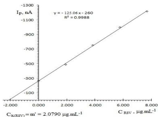
**Fig. 7: The standard addition curve for determination of RSV in Rosuvastatin-ElSaad (20 mg/tab.) using differential pulse polarographic analysis on mercury drop electrode with negative amplitude in di-sodium hydrogen orthophosphate buffer at pH 0.5**
