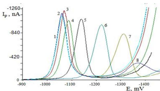
**Fig. 1: The effect of pH solution on the polarograms using DPPA at DME of RSV (9.63 µg.mL<sup>-1</sup>) at pH : 1- 0.1; 2- 0.2; 3- 0.5; 4- 1.0; 5- 2.0; 6- 3.0; 7- 4.0; 8- 5.0 (Purge gas N<sub>2</sub>, Purge time 200 s, Scan rate 6.6 mV/s, U. amplitude -60 mV, t. meas. 20 ms, t. pulse 60 ms, t. step 0.9 s, Temperature of solution 25± 5°C and buffer 0.075 mol.L<sup>-1</sup> di-Sodium hydrogen orthophosphate).**
