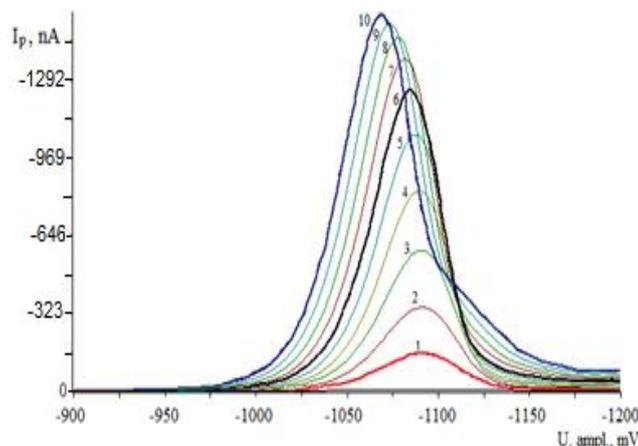
**Fig. 3: The effect of negative pulse amplitude (U ampl.) on the polarograms using DPPA at DME of RSV (9.63 µg.mL<sup>-1</sup>) at : 1) -10; 2) -20; 3) -30; 4) -40; 5) -50; 6) -60; 7) -70; 8) -80; 9) -90 and 10) -100 mV (Purge gas N<sub>2</sub>, Purge time 200 s, Scan rate 6.6 mV/s, pH=0.5, t. meas. 20 ms, t. pulse 60 ms, t. step 0.9 s, Temperature of solution 25± 5°C and buffer 0.075 mol.L<sup>-1</sup> di-Sodium hydrogen orthophosphate).**
