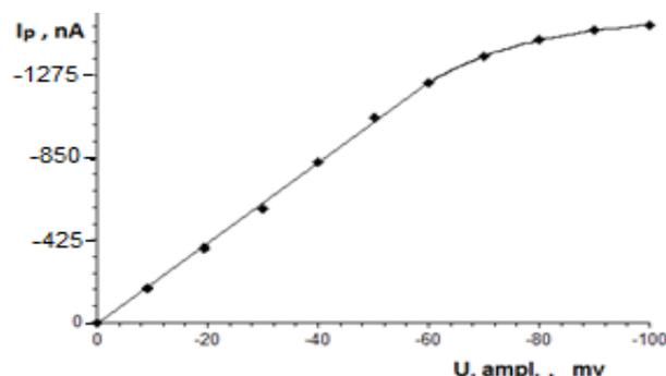
**Fig. 4: The effect of negative pulse amplitude (U ampl.) on  $I_p$  of RSV(9.63 µg.mL<sup>-1</sup>) using DPPA at DME (pH=0.5, Purge gas N<sub>2</sub>, Purge time 200 s, Scan rate 6.6 mV/s, t. meas. 20 ms, t. pulse 60 ms, t. step 0.9 s, Temperature of solution 25± 5°C and buffer 0.075 mol.L<sup>-1</sup> di-Sodium hydrogen orthophosphate).**
