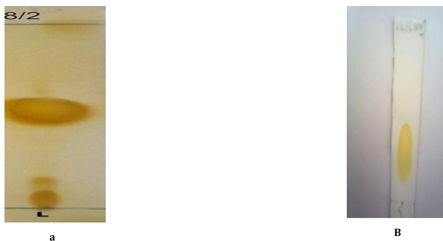
Fig. 2: TLC profile of esters (a and b: before and after chromatography column separation)
