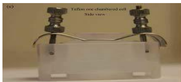
Fig.3: Nail support and incubation system: (a) Teflon one chamber diffusion cell components, (b) Teflon one-chamber diffusion cell top view, and (c) Teflon one chamber diffusion cell side view.
