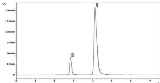
Fig. 5a: Chromatogram showing acid degradation of zotepine (an additional peak is observed at Rt 2.8 which is the peak of degraded product of zotepine)
