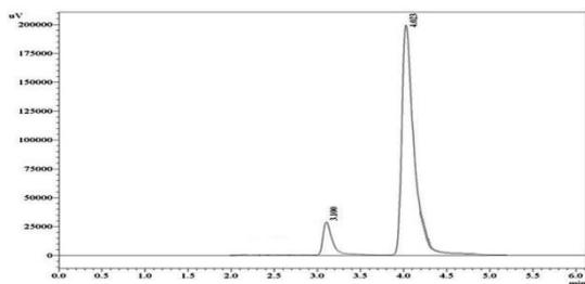
Fig. 5c: Chromatogram showing oxidative degradation of zotepine (an additional peak is observed at Rt 3.1 which is the peak of degraded product of zotepine.)
