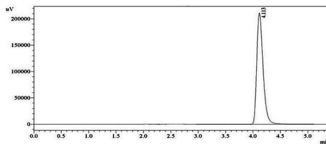
Fig. 3: Chromatogram of sample solution (marketed formulation)
