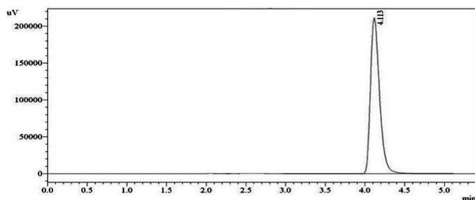
Fig. 2: Chromatogram showing estimation of zotepine (Rt 4.1)
