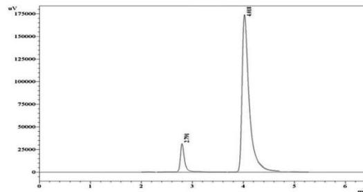
Fig. 5b: Chromatogram showing alkaline degradation of zotepine (an additional peak is observed at Rt 2.7 which is the peak of degraded product of zotepine)
