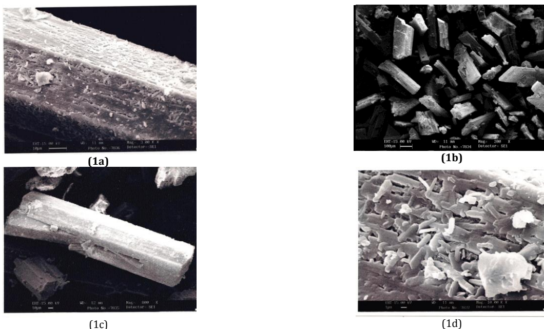
Fig. 1: SEM photomicrographs of; (1a) pure crystalline drug (1b) Fractured agglomerates (1c) Crystalline drug in the form of needles and has rough surface, (1d) Agglomerates has shown tube like structure and sintered crystals
