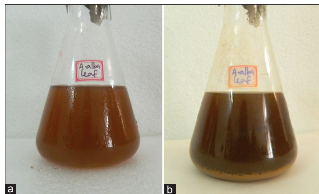
Fig. 2: (a) Leaf extract of Avicennia alba , (b) Brown solution of silver nanoparticles formed due to the reduction
